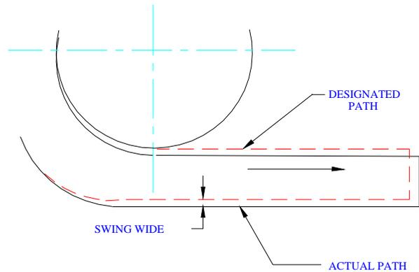
**Ashworth recommends a minimum swing wide clearance of 1 inch per foot of width [75 mm per meter of width] be built into all conveyors where the belt enters or exits a turn.**
