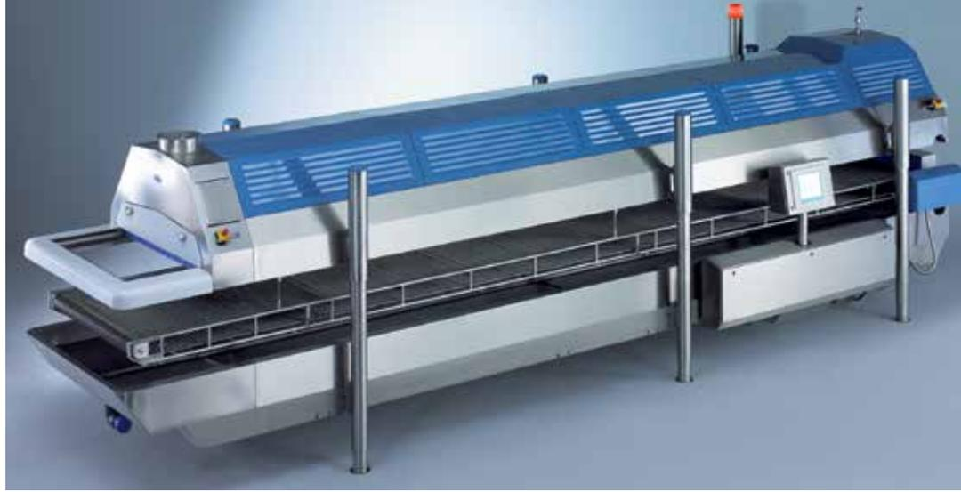
A cryogenic freezer can be installed before or after a mechanical freezer to boost performance. Linde
