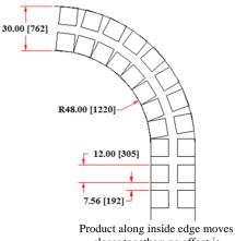
Product along inside edge moves closer together; no effect is observed on the product along outside edge. Loading: 1 in 1.63 product lengths.
