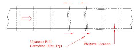
Rollers with frozen bearings have the opposite effect as the free turning roll. Consider the direction of oven expansion when setting roller positions. Expansion of the oven frame may bind a roller at baking temperature.
