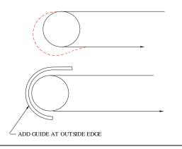
Also, the weight of the outside half of the belt causes the outside links to droop at the terminals. While this drooping is not an operating problem, it does not present a good appearance and may interfere with other equipment.
