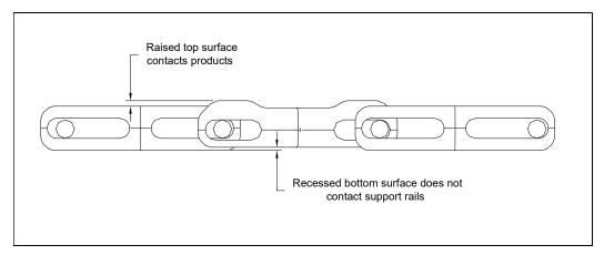
Figure 1. Cross-section of belt with friction module
