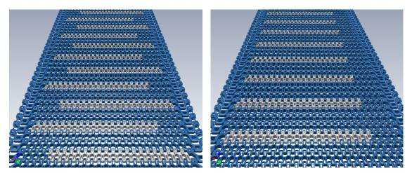
Figure 2. Odd and even pitch spacing (every 3rd-pitch on left and 4th-pitch on the right)
