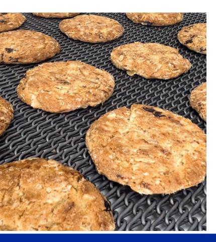
Made of carbon steel material, Ashworth's Z-Baking belt is available in several wire and mesh type configurations.
