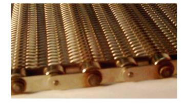
Length is generally the same as the overall width of the belt. Rod edges are welded, washer welded, brazed, washer brazed or drilled and cottered as specified. Winged rods are used to hold the chain sideplates in place when pin size rods are used with riveted hollow pin or cottered chain, located on every chain pitch.
